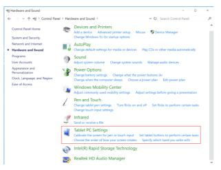
Step 4: Select " [ @Calibrate... " in the Tablet PC Settings window.
